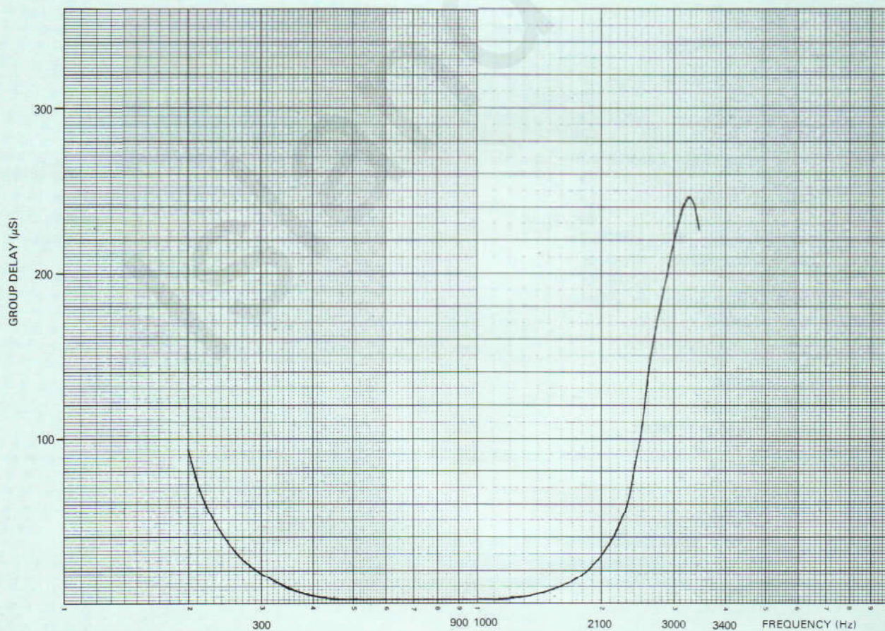
Fig. 5 FX306 Typical Group Delay Characteristics
