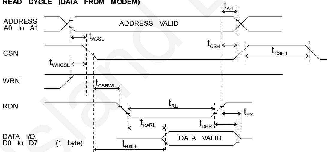
Figure 20  $\mu$ C Parallel Interface Timings
