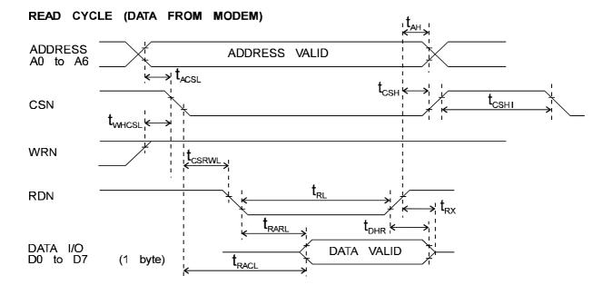
Figure 7  $\mu$ P Interface Timings
