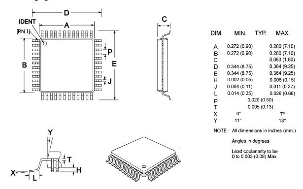
Figure 9 TQFP Mechanical Outline: Order as part no. FX949L4
