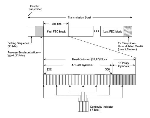
**Figure 5 Reverse Channel Transmission Structure**
