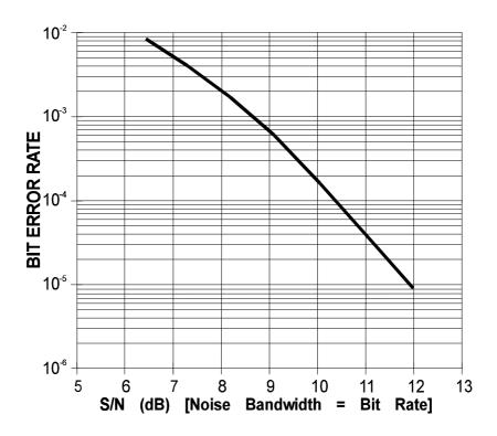
**Note:** This graph does not include the improvement in error rate that is achievable if error correction is included in the user's application software.
